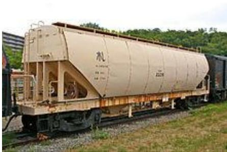
Hopper-bottomed railcars, such as this one from Japan, have made moving grain much faster and less labour-intensive.
