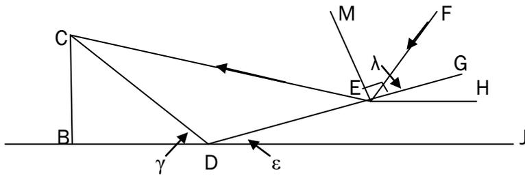
The panel CD now adjoins the reflector along DE (or there is a space, for rainwater). The panel angle to the horizontal is  $\gamma$ , the reflector angle is  $\epsilon$ , EH is a horizontal line and the light ray FE meeting the reflector at E makes an angle of  $\lambda$  with the continuation of DE to DG. Thus
