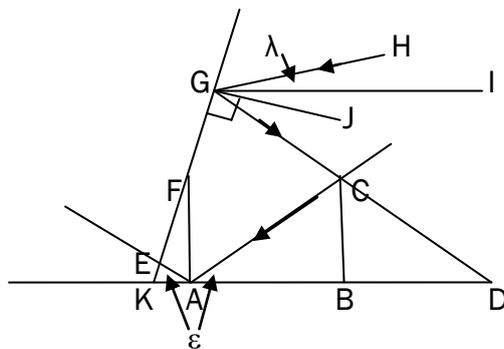
If in the diagram above CD is the panel and EG the reflector, at the winter solstice, a light ray along CA will meet the horizontal AB at an angle  $\epsilon$ . At the summer solstice, a light ray HG if at angle  $\lambda$  to the horizontal hits the panel after reflection at C.
