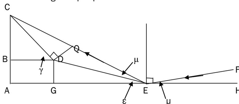
The panel at CD is now elevated by a height  $BA = DG$  above the flat roof, and the reflector along DE touches the flat roof at E. The edge ray FE continuing to C is now at an angle  $CEG = \mu + \varepsilon$  to the horizontal, and since angle  $\mu = 46.3^\circ$  and angle  $\gamma = 28.4^\circ$ , so  $\gamma < \mu$ , this is even worse than the horizontal case previously discussed.
