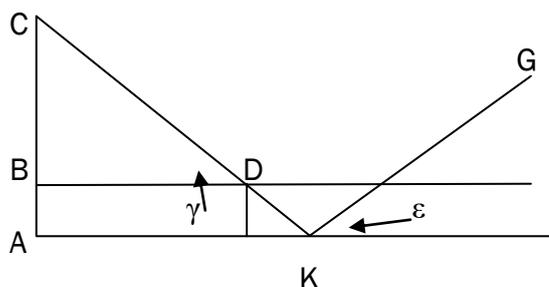
an imaginary continuation of CD meets the floor at K and the reflector is now along KG.
