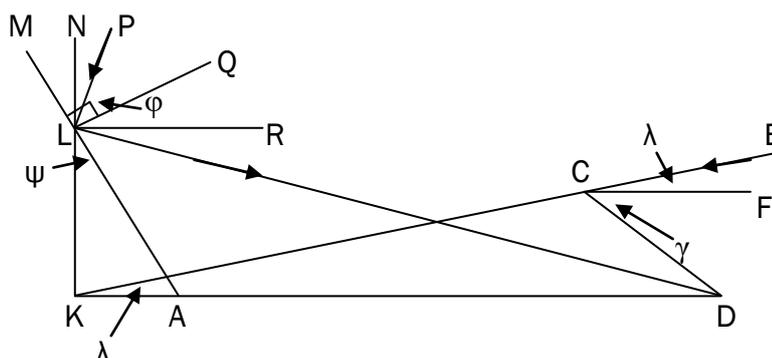
Let the panel be along CD with slope  $\gamma$ . At the winter solstice a light ray at angle  $\lambda = 15.8^\circ$  goes from C on the panel to K on the flat roof. KN is at right angles to KD. The reflector is aligned along AM at angle  $\psi$  to the vertical. KN meets AM at L. QL is at right angles to AL.
