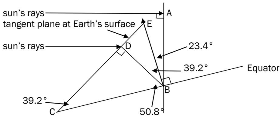
The Earth's orbital plane is called the ecliptic. In the diagram above the sun's rays meet the vertical to the plane of the ecliptic at right angles. B is at the centre of the Earth, and in this planar representation the line running through CB is in the plane defined by the equator. Brighton & Hove is represented at D, and the tangent plane at D (the flat roof!) is the line ED continued to C.
