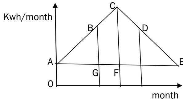
At which value is the area under AB equal to the area under BC? This should give an approximation to the average month for which the slope of the panel should be maximised. To do this we see that the area of triangle ACF is proportional to  $(AC)^2$ , and the area of triangle ABG, which has the same angles as triangle ACF, is proportional to  $(AB)^2$ . We have
