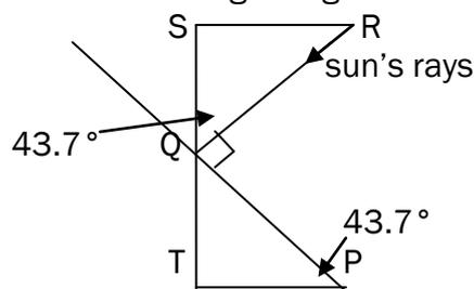
PQ is the panel. SQ is the vertical component of the sun's rays which are travelling along RQ. If the panel were horizontal, it would occupy part of PT and the total radiation on the panel would be reduced from a factor of 1 to  $\cos(\gamma_1) = \cos(43.7^\circ)$ .
