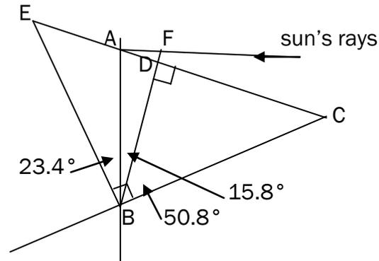
D is the location of Brighton & Hove and CD is a line tangent to the Earth's surface at D. B again depicts the Earth's centre, and BC represents a line going through the equatorial plane. BE at right angles to BC is the Earth's rotation axis, whereas BA is at right angles to the sun's rays.
