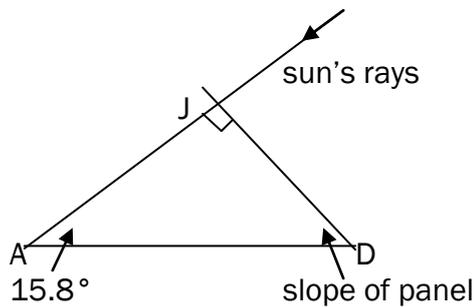
$$90^\circ + (66.6^\circ - \theta) + \text{angle JDA} = 180^\circ,$$
