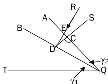
The adjusted panel is now at QA, and the original panel was at QB. Light rays hit QA along the old trajectory RE, and we want to find the vertical component to QA of this along SC. To do this we perform a similar calculation to the ones we have done previously to find that angle EDC is  $\gamma_2$ . Relative to a length or power value of ED = 1, the value of CD is  $\cos(\gamma_2)$ . The slope of the adjusted panel is  $\gamma_1 + \gamma_2 = 43.7^\circ + \gamma_2$ .
