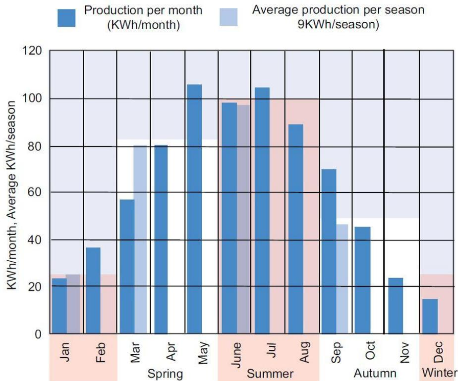
Figure 3. [MCS]. The chart above illustrates the seasonal variation in the energy production of solar panels. I believe that this is based on typical data on how solar panel systems are expected to perform.
