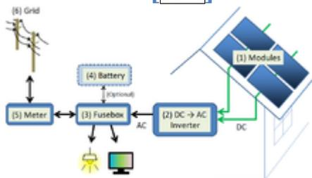
Simplified schematics of a grid-connected residential **photovoltaic** power system<sup>[1]</sup>
