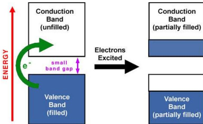
Add enough energy to an electron in the valence band of a semiconductor and it “jumps” to the conduction band. A free electron is an electron in the conduction band. In a PV panel a photon excites an electron out of the valence band into the conduction band. Free electrons can flow through the circuit, or in a process known as recombination drop back into the valence band. A built-in electrostatic field pushes the electron through the circuit.
