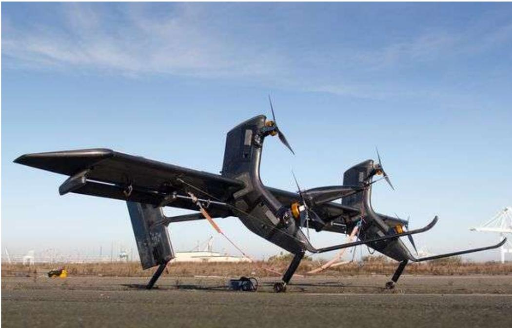
*Like the wing of a propeller plane without a cockpit, a Makani Airborne Wind Turbine stirs the air in a California field where it is being tested to capture high-altitude wind power.*
