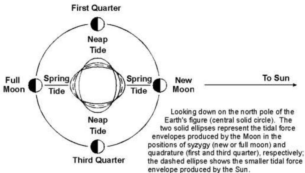
Shown in the diagram, much exaggerated, is the envelope of the oceans under the gravitational pull of the moon. As the moon circles the Earth, this causes the tides.
